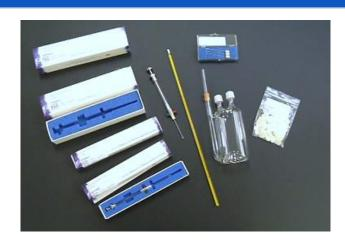
The PSA 10.555 Calibration Kit is used for the calibration of the PSA 10.525 Sir Galahad. The System includes a calibration vessel, thermometer, and a set of gas tight syringes. Hg vapour is drawn from the vessel and injected into the PSA Sir Galahad system. The user then tells the software the temperature and volume of Hg vapour injected and the software will then calculates the Hg vapour injected based on the vapour pressure of the Hg.
